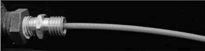
Slide the rubber grommet on the heat trace. Using a clean sharp blade cut a 2" slit along the heat trace outer jacket in the area where you are going to install the rubber grommet. Use extreme caution not to damage or cut the metal braid.
