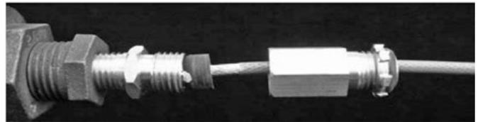
Completely tighten the union assembly compressing the rubber grommet making a water tight seal.
