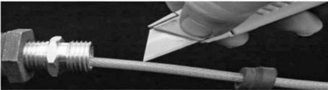
Carefully remove the overall jacket from the repair area. Use extreme caution not to damage or cut the metal braid.
