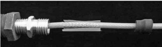
Apply Teflon paste to the exposed metal braid.
