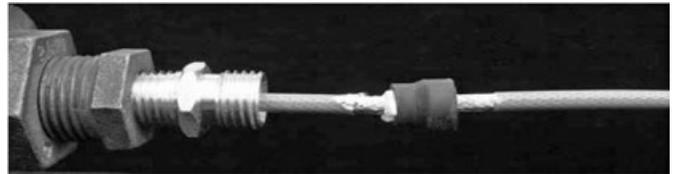
Reassemble the union assembly making sure the rubber grommet stays in place centered in the prepared area during this assembly.
