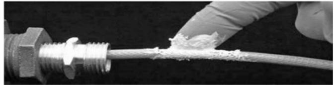
Slide the rubber grommet over the metal braid placing it in the center of the prepared area.
