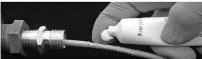
Massage the Teflon paste into the exposed metal braid. Make sure the paste covers the metal braid completely and fills all the holes in the metal braid as seen in Fig 1.
